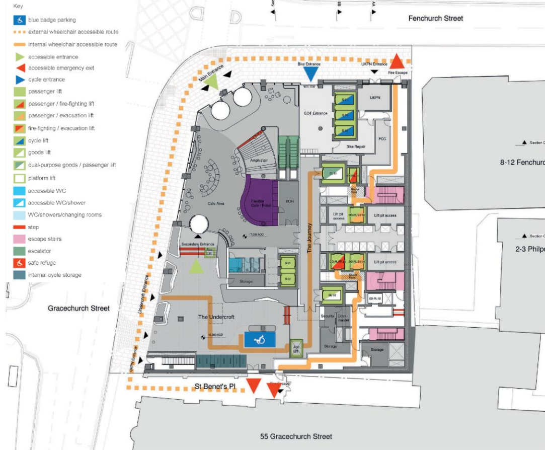
Fig.5 Ground Floor (ROUTE 1) Access Overlay
