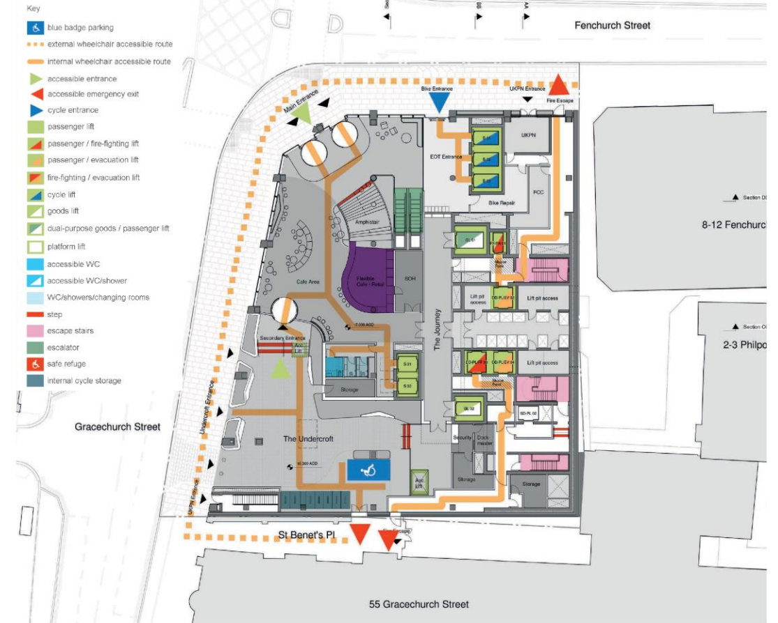
Fig.6 Ground Floor (ROUTE 2) Access Overlay
